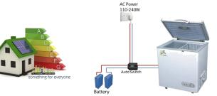
Battery Power with AC automatic Switch
